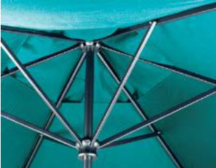
ARMS/RIBS The Portofino II arms are 1/2" x 7/8" non-tapered and are secured to the ribs with stainless steel nuts and bolts.
