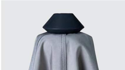
FINIAL The 1.5" x 3.5" finial has a 30% glass-filled nylon interior and HDPE outer shell in a dark grey color.
