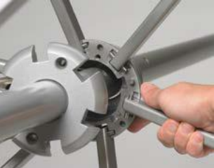
HUB The hub is cast aluminum and engineered for extra strength. It is split horizontally to encapsulate the stainless steel direct connect pin assembly. Two screws secure the hub together.
