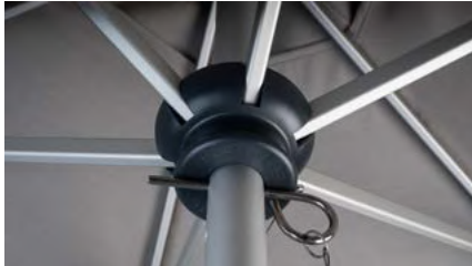
HUB The hub has a 30% glass-filled nylon interior and HDPE outer shell in a dark grey color. It is split horizontally to encapsulate the stainless steel connecting hardware. Six screws secure the hub together.
