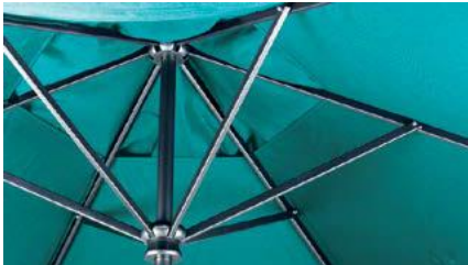
ARMS/RIBS The Portofino arms are 3/4" x 1-3/8" non-tapered and are secured to the ribs with stainless steel nuts and bolts.
