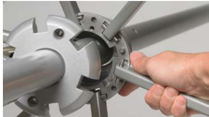
HUB The hub is cast aluminum and engineered for extra strength. It is split horizontally to encapsulate the stainless steel direct connect pin assembly. Two screws secure the hub together.
