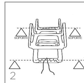
Start stringing the elastic cord through both eyelets of the fabric and the holes of the resin frame. Start from the middle of the cross bar of the adjustable back of the chaise and make two equal ends of cord.
