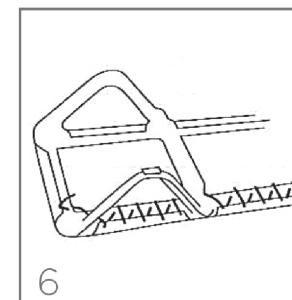
Keep stringing both sides of the bottom part of the Sling Chaise simultaneously as before. Pull and stretch both ends of the cord as soon as you reach the bottom corners of the Sling Chaise.
