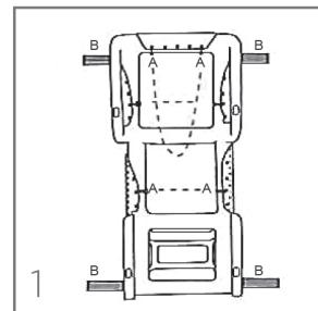
Place the Sling Chaise upside down on two table height trestles, with the Sling Chaise back opened in the highest position. Stretch and hold the fabric in proper place. Ideally, using bungee cords (not supplied).
