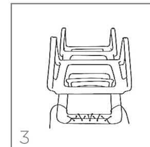
String the fabric simultaneously along both sides of the cross bar of the back of the Sling Chaise. Upon reaching the corners of the back top, pull and stretch both ends of the cord on either side of the Sling Chaise.
