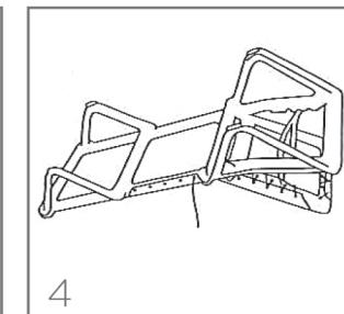
String the fabric on both sides of the chaise back simultaneously until you reach the back hinge. Pull and stretch both ends of the cord on either side of the Sling Chaise at the same time. Remove the bungee cords under the back.
