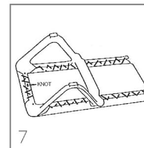
Complete the threading of the bottom traverse of the Sling Chaise. Pull and stretch both ends of the cord. Tie a knot at both ends close to the holes near the middle of the bottom traverse of the Sling Chaise frame.
